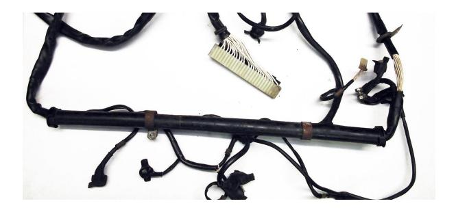
It is required so that we can re-use the original BMW split conduit with its associated collars and four original BMW grommets including any associated plates, all of which are no longer available to us.
